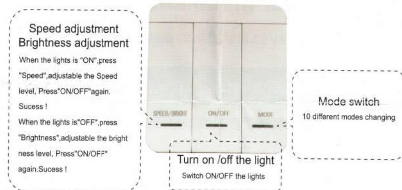
**Reset function:** press the "mode key" and "speed key" at the same time in the turn on light state to restore the factory default mode.
