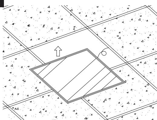
2. Put up the panel onto the ceiling
