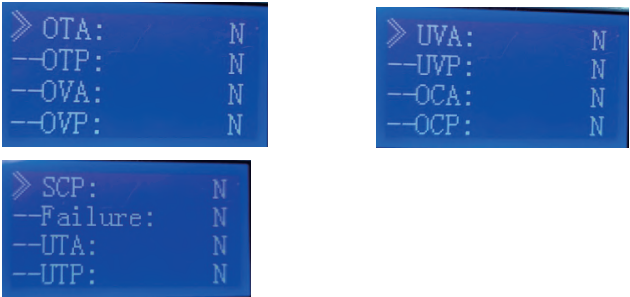
Figure 1-9 BMS State Parameters
