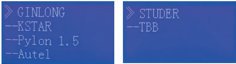
Figure 1-12 CAN Protocol setupinterface
