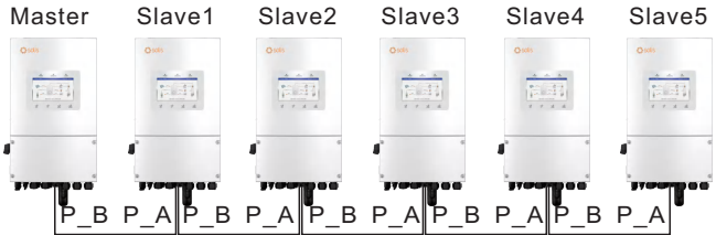
Figure 3.24 Parallel Terminal Connection
