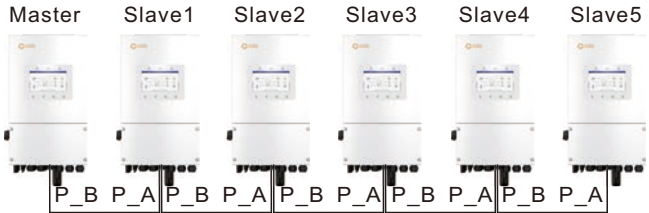
Figure 3.24 Parallel Terminal Connection
